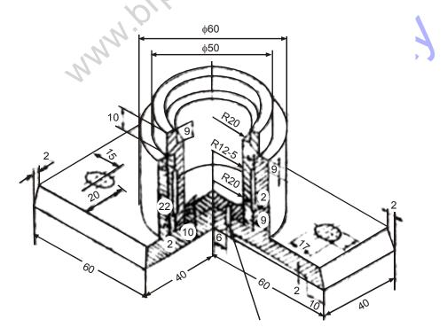
9. Figure below snows manges, keys and snams to be connected in a flange coupling, Assemble and draw elevation and side view in full. Note that nuts and bolts are to be added.
